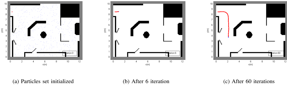
Fig. 10: Monte Carlo Localization algorithm experiments in map 2.
